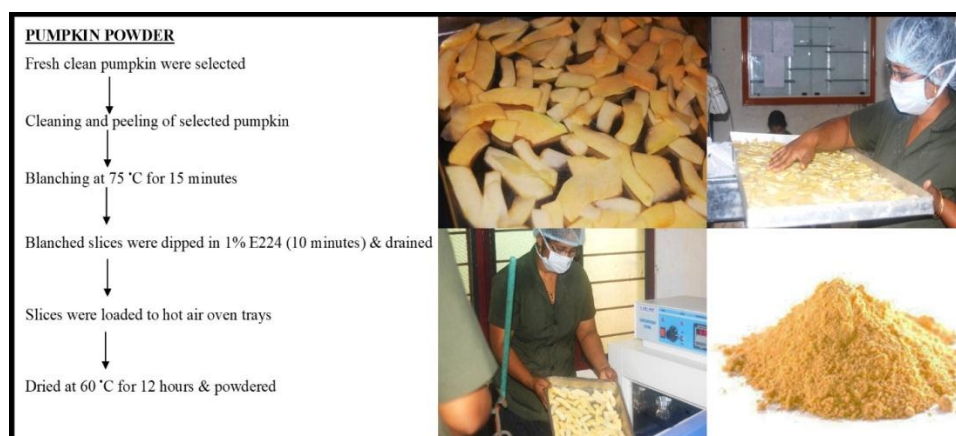
Fig. 4: production process for making pumpkin powder
